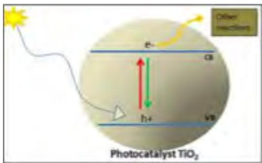
*Figure 1. Electron ( $e^-$ ) is excited to CB (red arrow), generating a hole ( $h^+$ ), where it can either be utilized in another reaction (yellow arrow), or it recombines (green arrow), returning to the valence band.*
