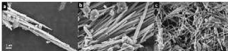
Figure 4. Three calcination temperatures were explored in the synthesis using phosphoric acid in a 2M concentration (a. 500 °C: 5 hours, b. 650 °C: 12 hours, c. 800 °C: 5 hours).
