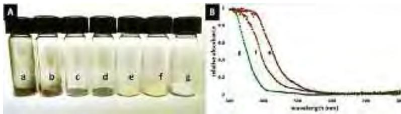
Figure 8. A: A digital image showing the different color powders synthesized with varying acids (a. pure TiN, b. HCl-2M, c. PA-2M, d. NA-1M, e. NA-2M, f. NA-4M, g. commercial P25- $\text{TiO}_2$ ). B: UV-visible diffuse reflectance spectra of selected samples (g. P25- $\text{TiO}_2$ , f. NA-4M, e. NA-2M).
