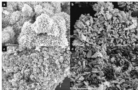
*Figure 3. Four acid concentrations were explored in the synthesis using nitric acid (a. 1M, b. 2M, c. 3M, d. 4M).*
