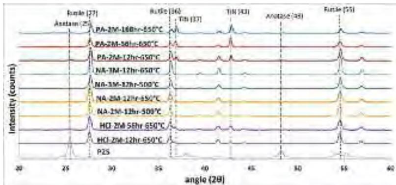
Figure 7. XRD analysis of samples confirm a mostly rutile composition with some peaks matching those of the precursor titanium nitride (TiN).
