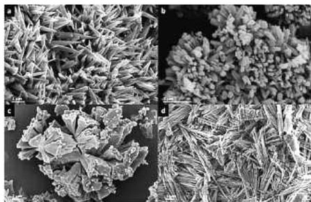
*Figure 2. Four acids at a final concentration of 2M were explored in the synthesis of  $\text{TiO}_2$  (a. hydrochloric acid, b. nitric acid, c. sulfuric acid, d. phosphoric acid).*
