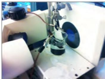
**FIGURE 2:** *Setup for Etching Pt-Ir Tips*
