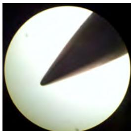
**FIGURE 5:** *Fine Etched Tip After Both Methods (1000x)*
