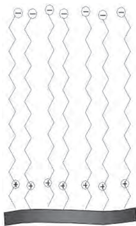
Figure 1: Diagram of the zwitterionic stationary phase Obelisc R. Figure adapted from Sielc Obelisc web material. ( http://www.sielc.com/Products_Obelisc.html , accessed Sep 2010)
