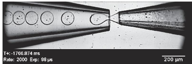
**Figure 3.** Brightfield image of tapered ends of the glass capillaries forming double emulsions. The dark spots inside the double emulsions are polystyrene particles.
