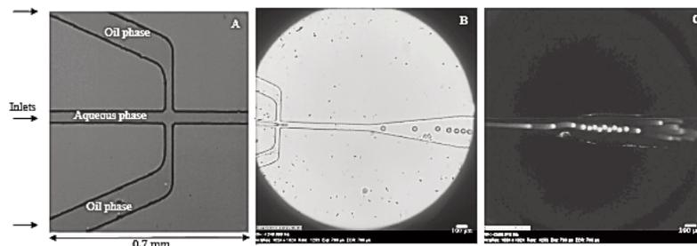
**Figure 1.** (A) Labels for the direction of flow of the oil and aqueous phase from the inlets. (B) Brightfield image of the formation of inverted emulsion droplets containing 200mM sucrose, 100mM Bis-Tris, 0.7mg/mL sulforhodamine B, and silica Janus particles. (C) Laser-induced fluorescence image of the formed inverted emulsion. Figures 1B and 1C are viewed from a 10x objective.
