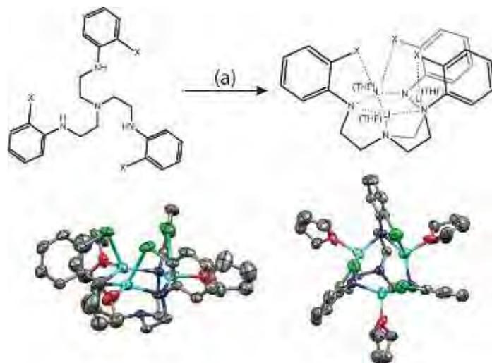
**Figure 4.** The lithiation of the TREN ligands, where (a) is *n*-butyllithium or *t*-butyllithium. The solid state structure of the trilitium complex of the TREN formed from 2-chloroaniline is shown with a side view (left) and a top view (right).
