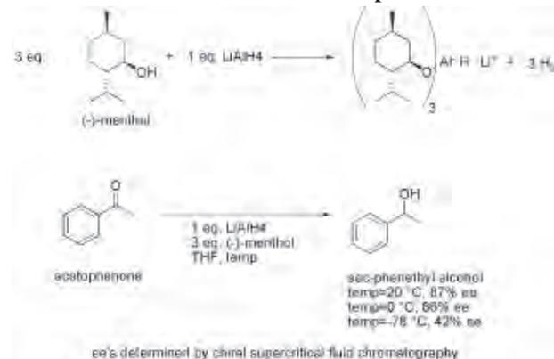
lithium aluminum hydride (LiAlH<sub>4</sub>), a common reducing agent. Similar methodologies are known but not well-developed.<sup>i, ii</sup> In the reaction mixture, (-)-menthol reacts with LiAlH<sub>4</sub> to make lithium tri-menthyloxyaluminum hydride, which then reduces acetophenone to *sec*-phenethyl alcohol. In our experiments, one enantiomer of *sec*-phenethyl alcohol was obtained in 87% enantiomeric excess (ee). Decreased temperature lowers the selectivity of the reaction (Scheme 2)
