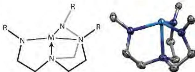
**Figure 1.** The generic structure of the TREN ligand set, showing a metal bound in the tetradentate, tripodal tris(amido)amine binding pocket.
